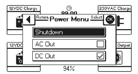
To turn on both 230VAC and 12VDC output press . If only 230VAC or 12VDC is needed select either "AC Out" or "DC Out" and press . The power menu for choosing 230VAC and/or 12VDC can always be accessed by pressing the power button .
